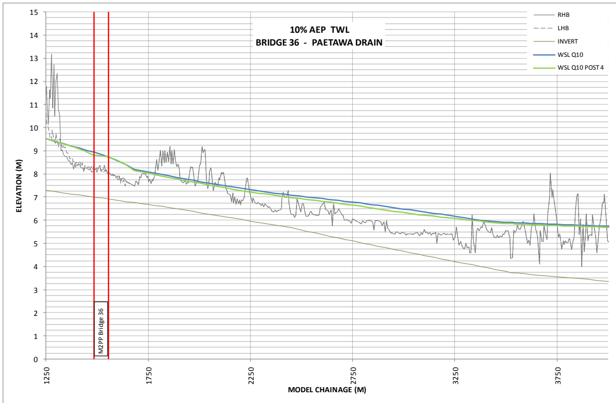
Figure 16 Paetawa Drain- 10%AEP Top Water Level
