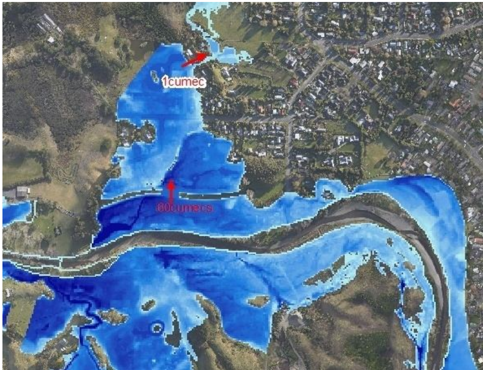
Figure D.2 Kauri Puriri stopbank breach peak flood depths and flows (Q100CC)
