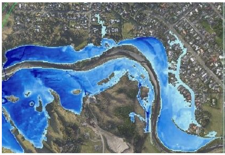
Figure D.7 Jim Cooke Park stopbank breach (downstream site) peak flood depths (Q200CC)
