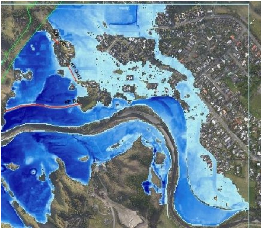
Figure D.3 Kauri Puriri stopbank breach peak flood depths (Q2500CC)
