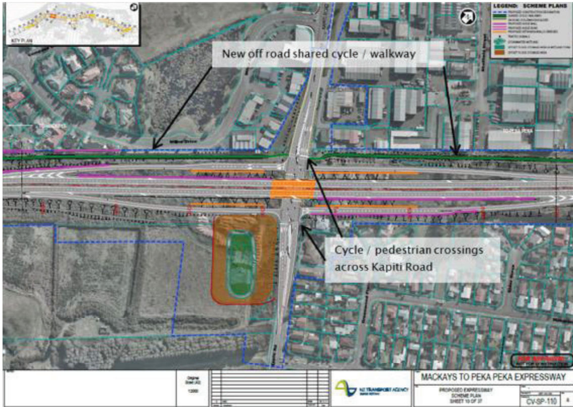
Figure 6.2: Kāpiti Road Cycle / Pedestrian Facilities
