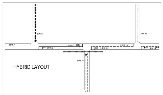
Figure 5.2.3 - Hybrid Lane Arrangement
