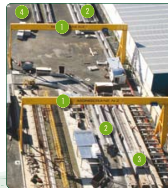
Gantry cranes (1) are used to lift beams (2) from the mould (3) and around the storage area (4) at the projects precast yard in Takanini.
