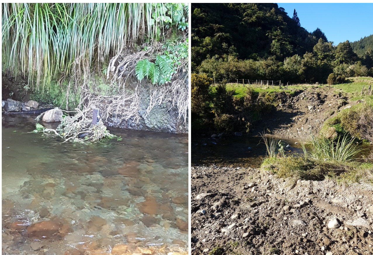
Figure 3.3: Debris trapped around the base of the turbidity sensor in Waitohu Stream (left) and a ford constructed approximately 50m upstream of the monitoring site (right).
