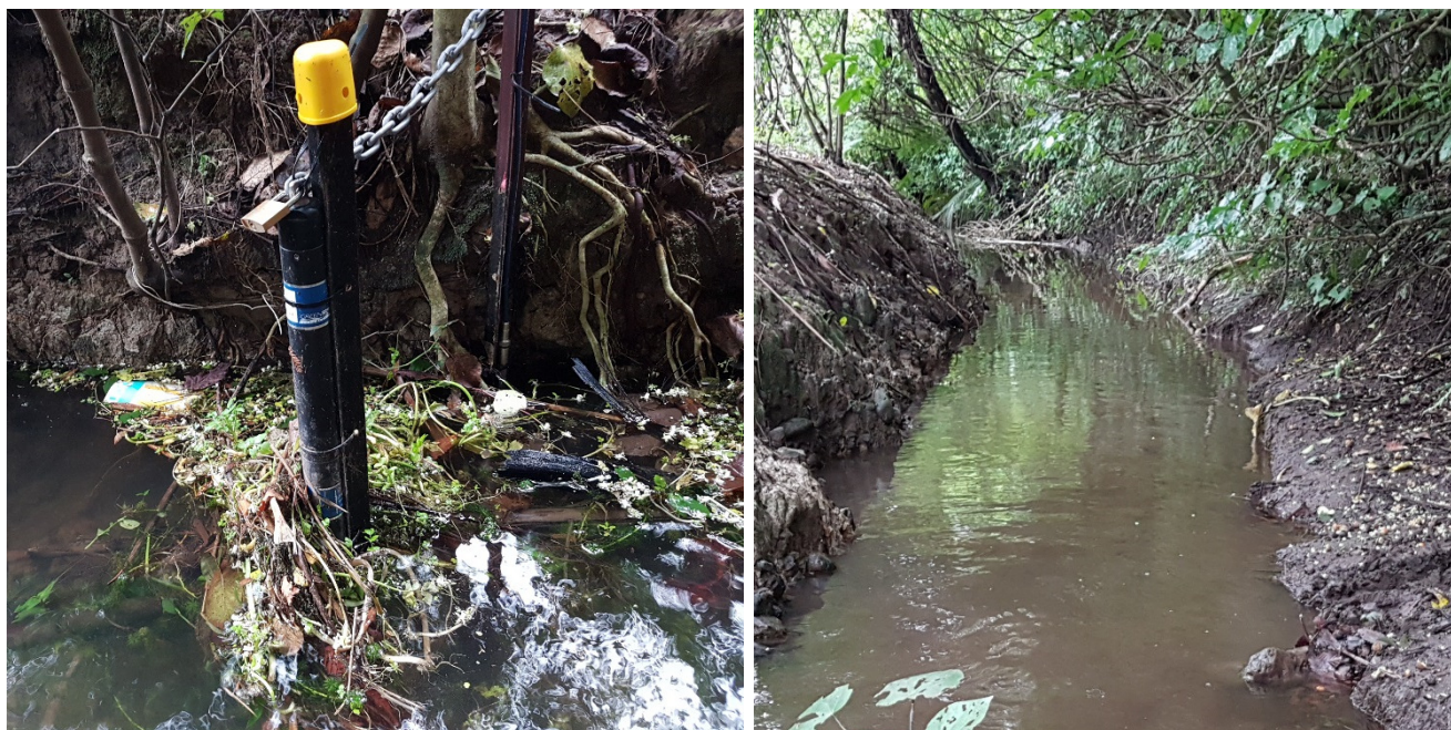
Figure 3.4: Trapping of debris around the turbidity and water level recorder in the Mangapouri Stream (left). Increased water level as a result of the backwater effect of a fallen tree in the stream (right).
