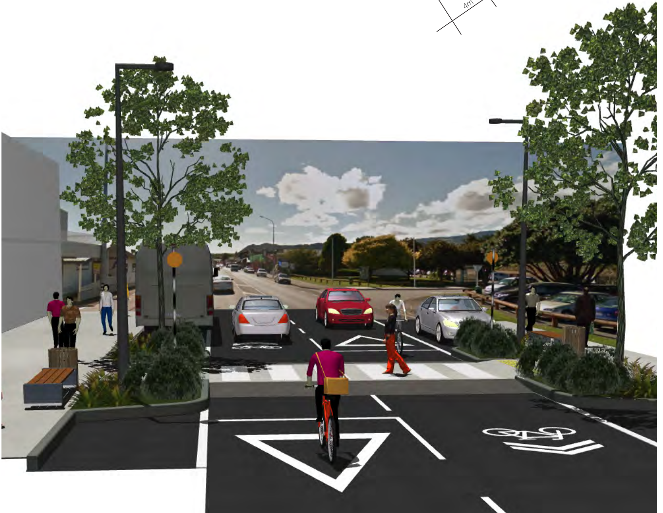
Figure 52. Ōtaki View D Raised Crossing Street View
