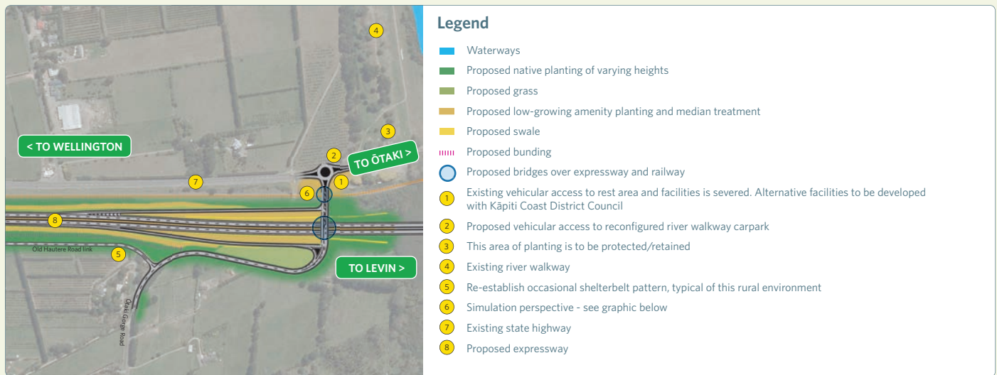
South Ōtaki interchange - indicative mitigation shown
