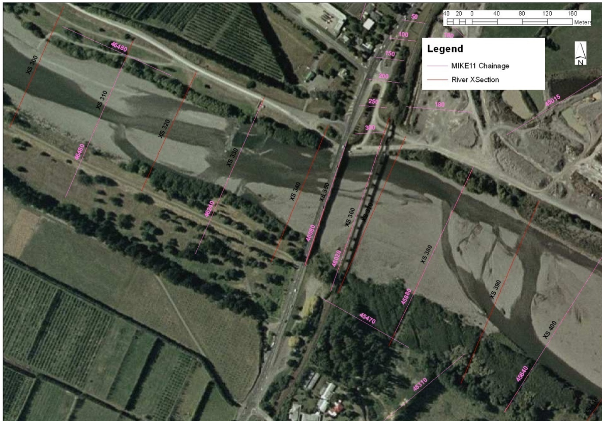
Figure 4-8: GWRC surveyed river cross-sections on Otaki River near expressway crossing
