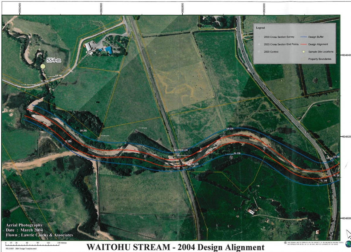
Figure 4-12: GWRC’s design alignment and buffer zone for Waitohu Stream downstream of existing SH1 Bridge
