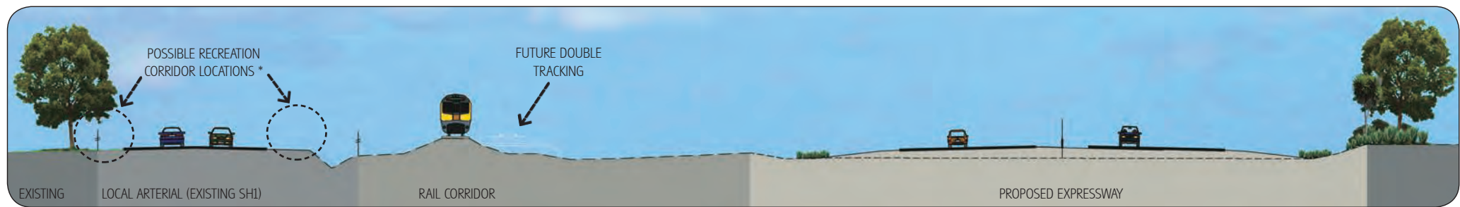
Figure 16. Typical Cross Section North of Te Horo
