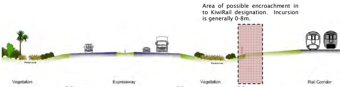
Figure 3.4. Typical Cross Section north of Te Horo
