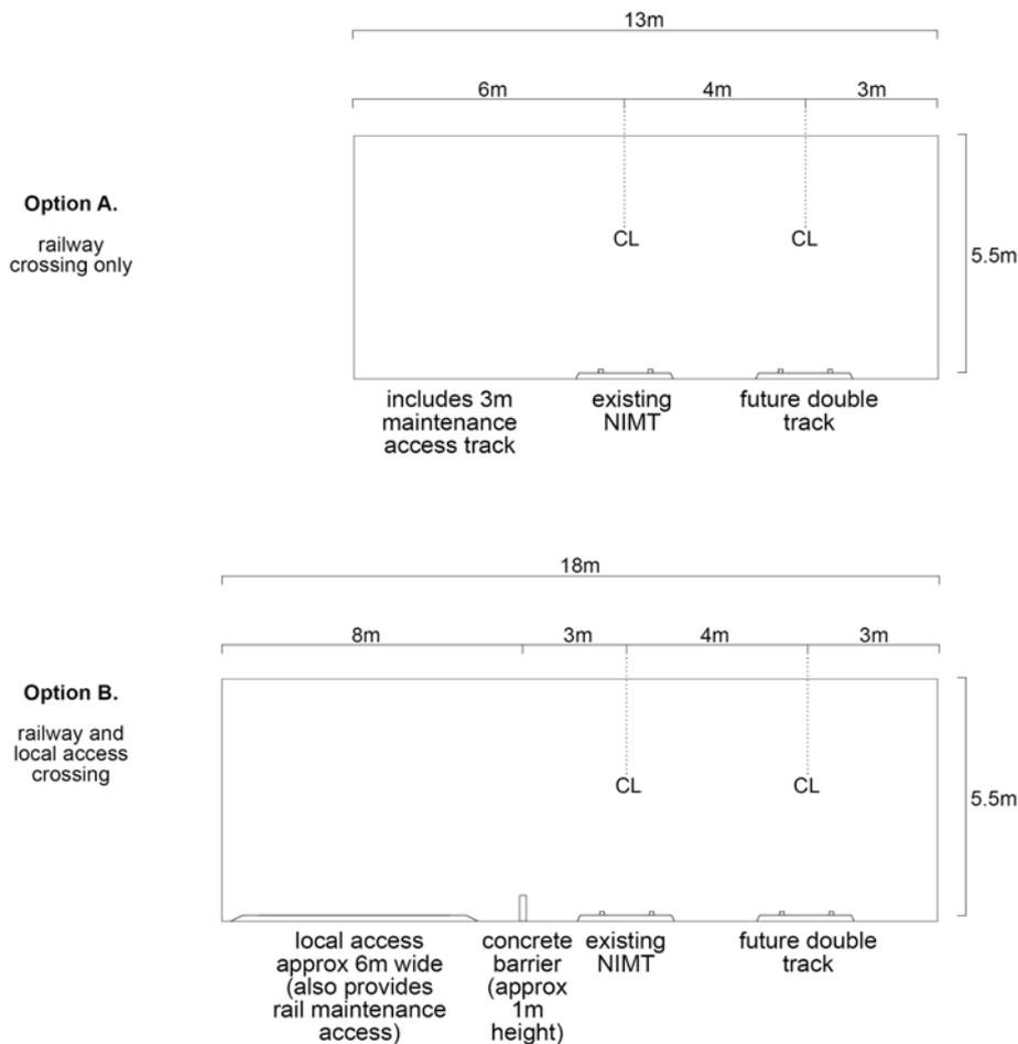
**Figure 3.2. Minimum clearances under structure at Mary Crest.**
