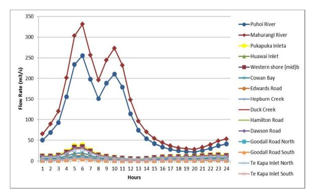
Figure 8: Hydrograph used as inputs for the 50 year (ARI) rainfall event scenario.
