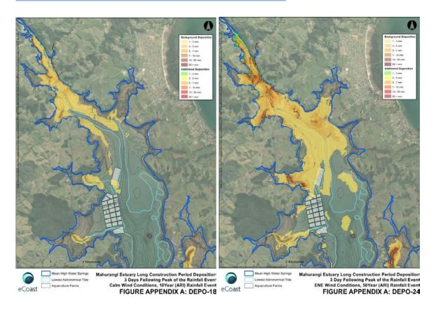
Figure 16: Predicted impacts of the additional sediment associated with the peak open earthworks in the long construction programme in the Mahurangi Estuary in the 10 and 50 year ARI sediment load scenarios.
