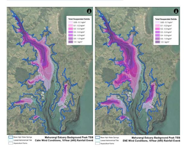
Figure 10: Comparison of background peak total suspended sediment in the Mahurangi Estuary in the 10 year sediment load scenario under the two different wind conditions.
