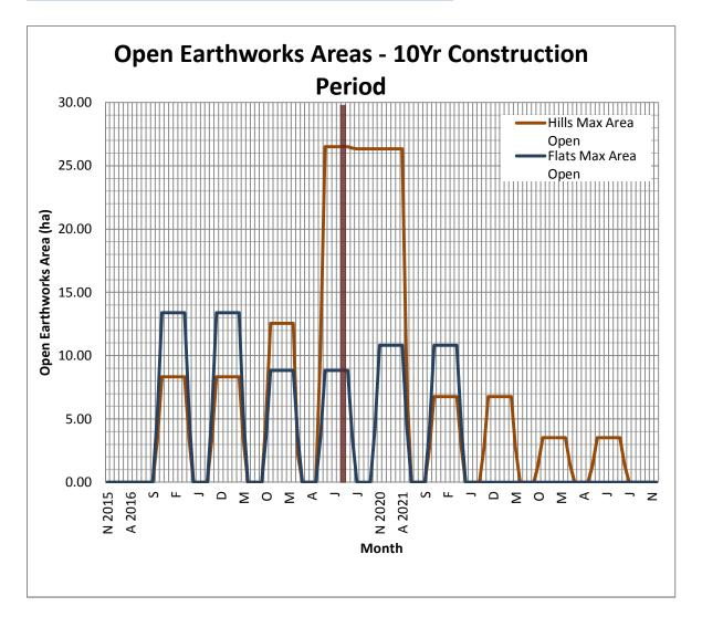
Figure 3: Areas of open earthworks in the Mahurangi Catchment based on a 10 year construction programme.
