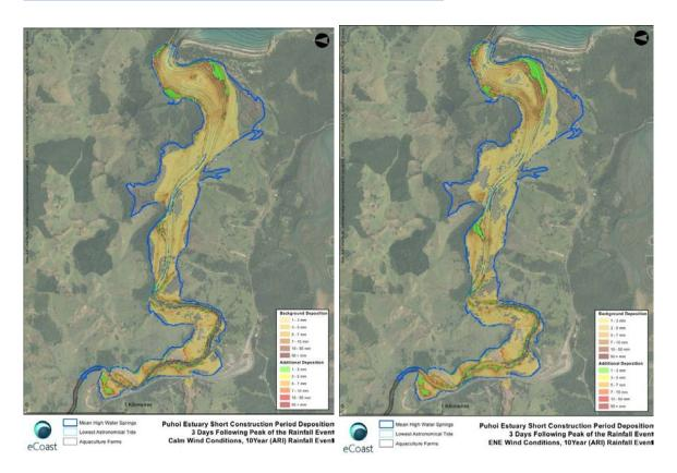
Figure 21: Predicted impacts of the additional sediment associated with the peak open earthworks in the short construction programme in the P**ū**hoi Estuary during a 10 year (ARI) sediment load scenario under calm and ENE wind conditions.
