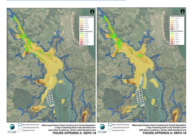
Figure 15: Predicted impacts of the additional sediment associated with the peak open earthworks in the short construction programme in the Mahurangi Estuary during a 50 year ARI sediment load scenario under calm and ENE wind conditions.
