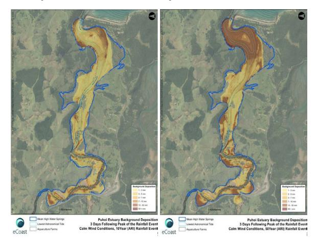
Figure 19: Background deposition in the P**ū**hoi Estuary in the 10 and 50 year sediment load scenarios.
