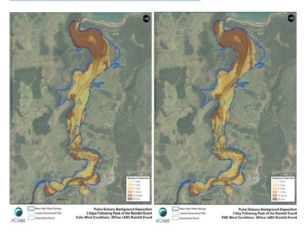
Figure 20: Background deposition in the P**ū**hoi Estuary in the 50 year sediment load scenario under calm and ENE wind conditions.
