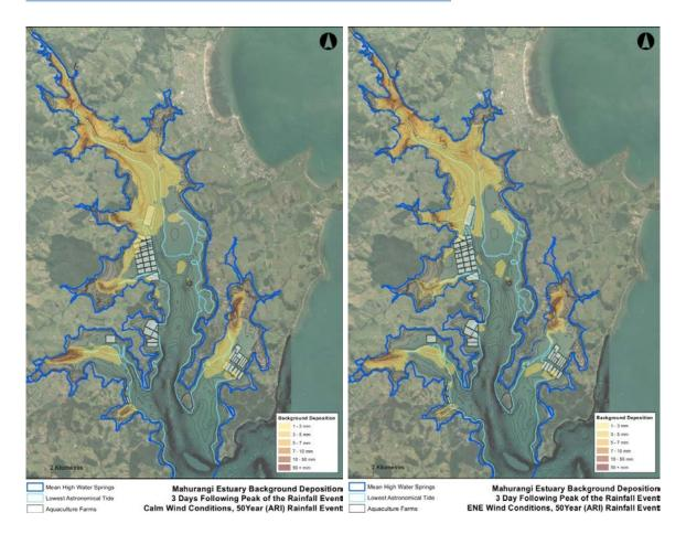
Figure 13: Background deposition in the Mahurangi Estuary in the 50 year sediment load scenario under calm and ENE wind conditions.
