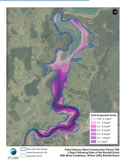
Figure 18: Background total suspended sediment in the P**ū**hoi Estuary 1 day after peak of the 50 year sediment load scenario including the 9m/s ENE wind.
