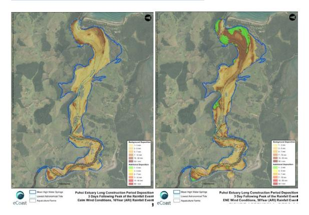
Figure 23: Predicted impacts of the additional sediment associated with the peak open earthworks in the long construction programme in the  $P\bar{u}$ hoi Estuary in the 10 and 50 year (ARI) sediment load scenarios.
