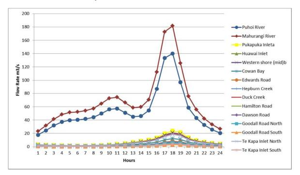
Figure 7: Hydrograph used as inputs for the 10 year (ARI) rainfall event scenario.
