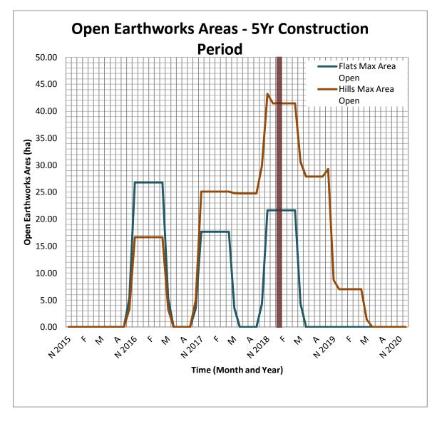
Figure 2: Areas of open earthworks in the Mahurangi Catchment based on a 5 year construction programme.
