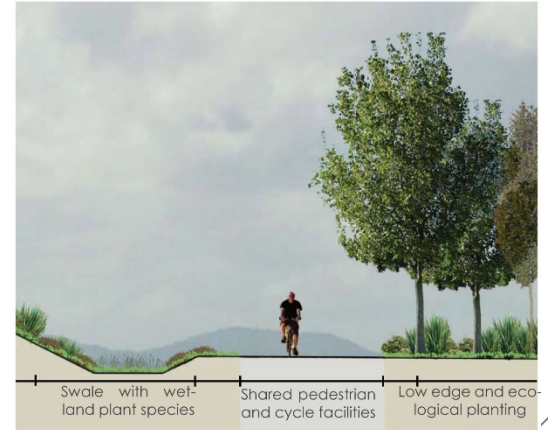
Swale integrated with pedestrian and cycle facilities
