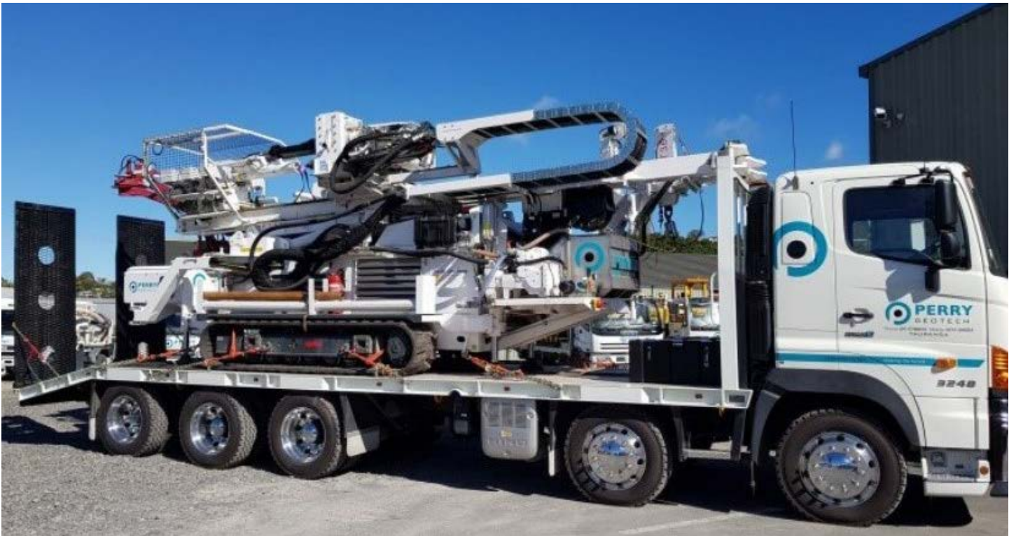
Machine boreholes are drilled using a rig.
