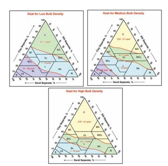
Figure O2 Saturated Hydraulic Conductivity
