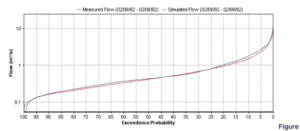
K.5 Porirua Stream: Observed and Simulated Flow Duration Curves
