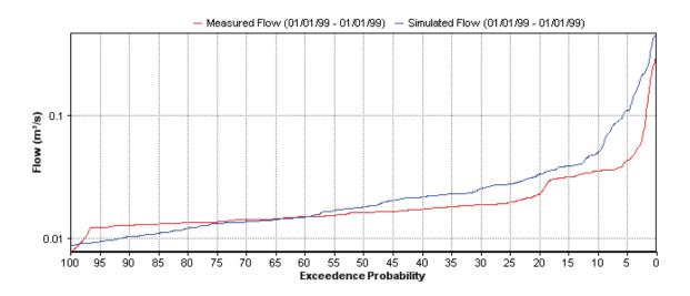
Figure K.8 Wainui Stream: Observed and Simulated Flow Duration Curves
