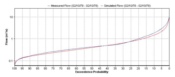
Figure K.6 Pauatahanui Stream: Observed and Simulated Flow Duration Curves
