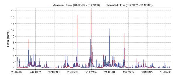
Figure K.4 Horokiri Stream: Observed and Simulated Hydrographs
