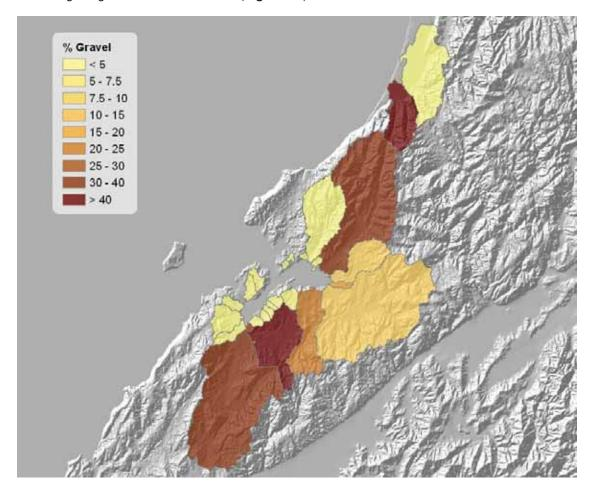
Figure N3 Average Gravel Content from Catchments Based on Test Pits
