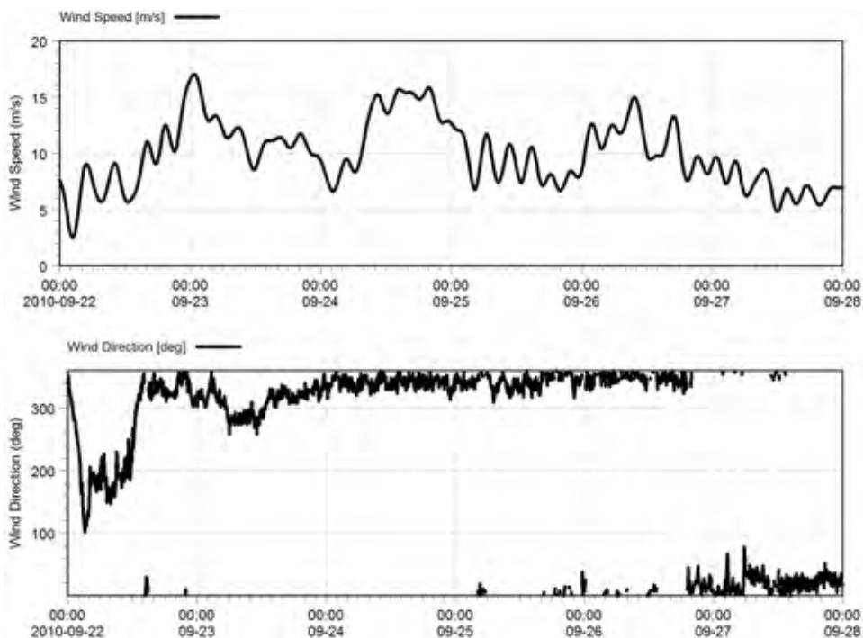
Figure V54 Wind Speed (top) and Wind Direction (bottom) Observed in Pauatahanui Inlet for First Sediment Transport Calibration Period
