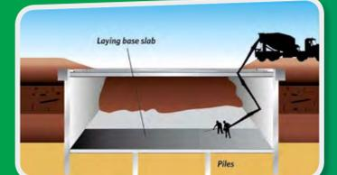
The floor of the tunnel is built, and anchored into the bedrock below.
