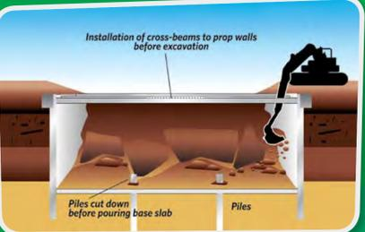
Excavators remove the dirt and rock from between the walls.
