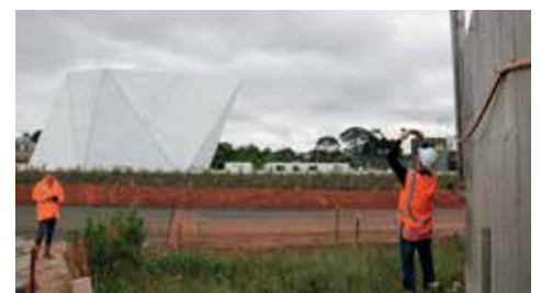
Acoustic testing outside at the property boundary.
