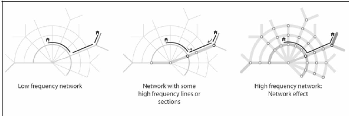
Figure 3.2 illustrates the network effect. The network effect centres on frequency and coverage of the public transport system. If services operate at low frequency, waiting times are long and if transfers are required it may not be the most desirable transport option. By contrast, higher frequency lines offer a system that competes with the car (Nielsen and Lange 2008).
