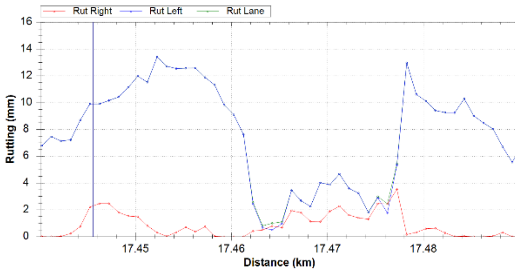
Figure C.39 Hawkeye rut measurement for mill and AC inlay at 16- month inspection SH27-RS46-17445-17485 (decreasing side)
