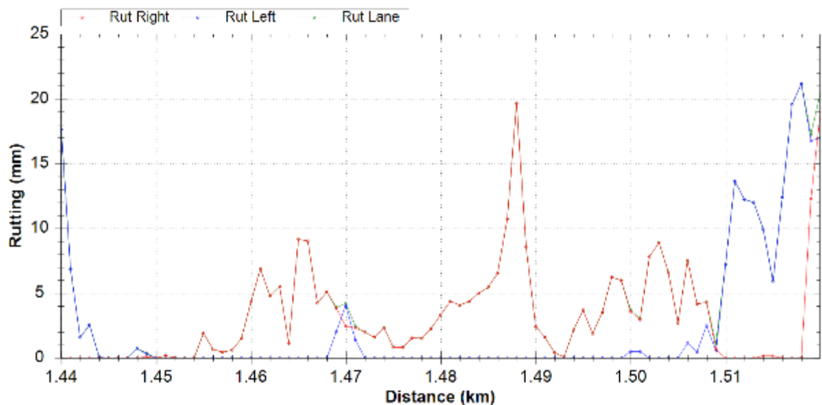
Figure C.7 Hawkeye rut measurement for 1.5% cement in- situ stabilisation at 16- month inspection (1.50 to 1.52 km)
