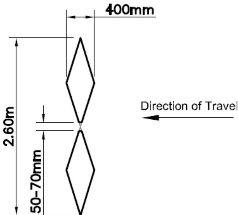
**Figure 23: Revised ZELT loop layout on Riccarton Road**
