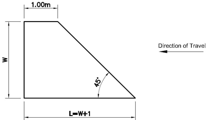
**Figure 4: Bicycle recorder loop configuration**
