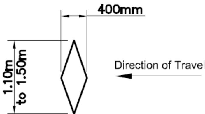
**Figure 9: ZELT loop configuration**
