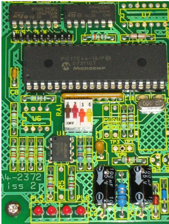
**Figure 3: Switch configuration in the Bicycle Recorder**
