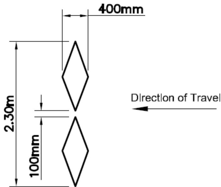
**Figure 16: ZELT loop layout for Riccarton Road, Dyers Pass Road and Sparks Road**
