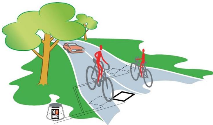
**Figure 1: Eco-Counter's ZELT inductive loops**
