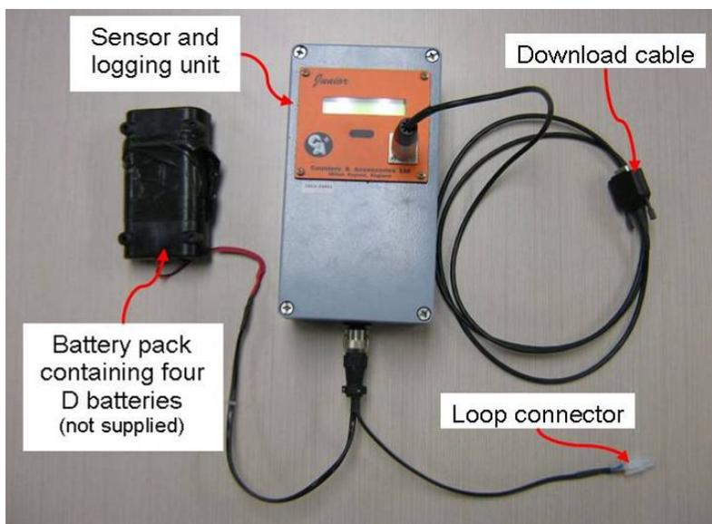
**Figure 2: Bicycle recorder components**
