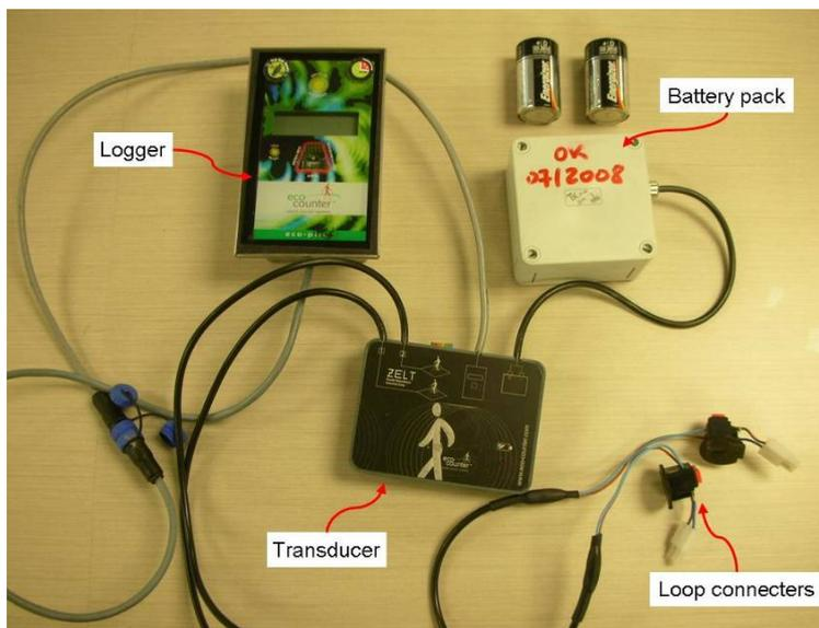
**Figure 7: ZELT eco-twin components**
