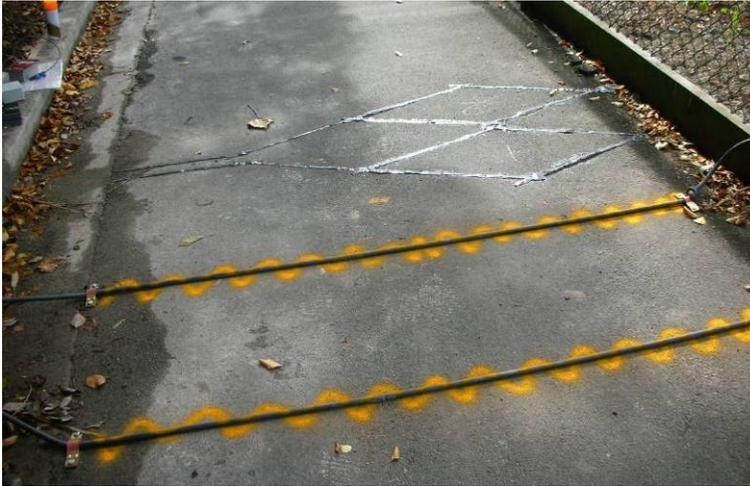
**Figure 13: ZELT loop and eco-tubes on the railway cycleway**
