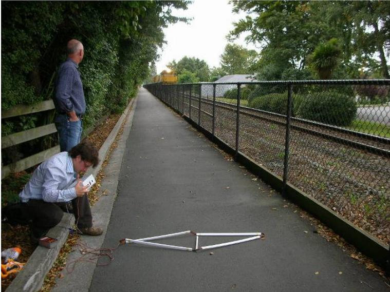
**Figure 10: ZELT test loop and white box**
