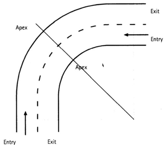
Vehicle rollovers normally occur between the apex and the exit of a corner as a result of excessive speed or braking. When towing a trailer, the prime mover must pull the trailer through the bend, not be pushed by it. This can only be achieved with the cornering technique. Cornering stability will be improved, and the effects of centrifugal force reduced, if the correct cornering line is also applied.
