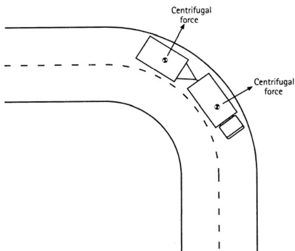
Centrifugal force is affected by the vehicle speed and the angle of turn. In other words, the faster the vehicle is going and/or the tighter the turn, the more likely the driver is to lose control of the vehicle and for it to roll over.
