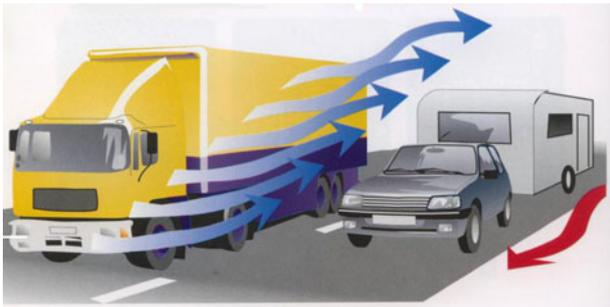
Remember also that your vehicle will generate its own wind as it moves along the road. The faster you go, the greater the wind forces generated will be. These forces can be sufficient to blow motorcyclists over and buffet other vehicles to a point that the driver loses control, so you need to be considerate of other road users and slow down.
