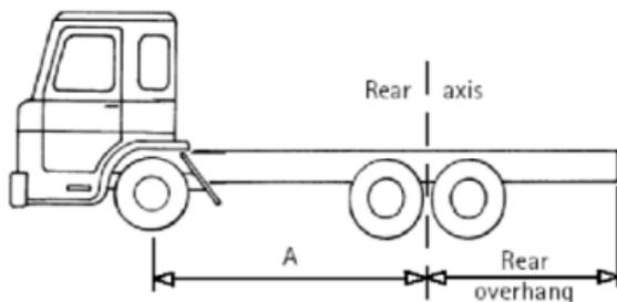
Rear overhang means the distance from the rear axis to the rear of the vehicle or its load, whichever is greater. For a heavy rigid vehicle, in which the rearmost axle is a non-steering axle, the maximum rear overhang is either 4 metres or 70 percent of
