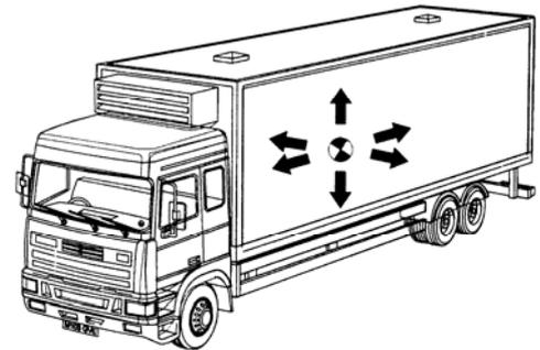
If the load is not balanced correctly along its length, wheel lock-up during braking becomes a distinct possibility. When wheel lock-up occurs, the vehicle loses steering control.
