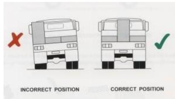
Heavy items should be placed to the bottom of the load so that the CG remains as low as possible.
