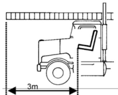
When front overhang is excessive, the part of the load that is overhanging the vehicle will travel in a wider arc than that taken by
