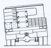
Incorrect: Load improperly balanced
