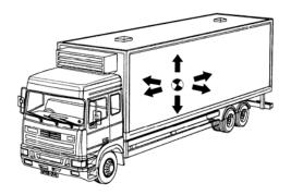
If the load is not balanced correctly along its length, wheel lock-up during braking becomes a distinct possibility. When wheel lock-up occurs the vehicle looses steering control.
