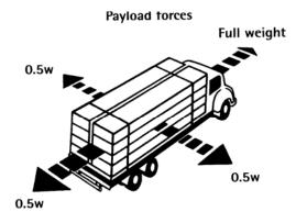
requirements, as shown in the Truck loading code, rests with the driver. The responsibility starts at the time of loading. Placing loads that increase the height of the vehicle's CG or shifts it off-centre (closer to one side) will reduce the vehicle's stability and dramatically affect its handling.
