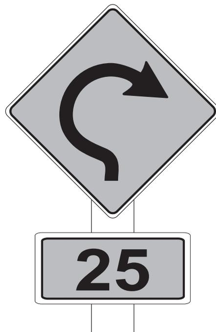
The speed squared effect means the difference in speed between 0.22g and 0.35g can be small. For example, a truck driving through a curve with a 25km/h speed advisory sign at the posted speed would experience a 0.22g lateral acceleration. If the truck travelled through the curve at 31.5km/h, the lateral acceleration would be 0.35g, only a 6.5km/h difference.
