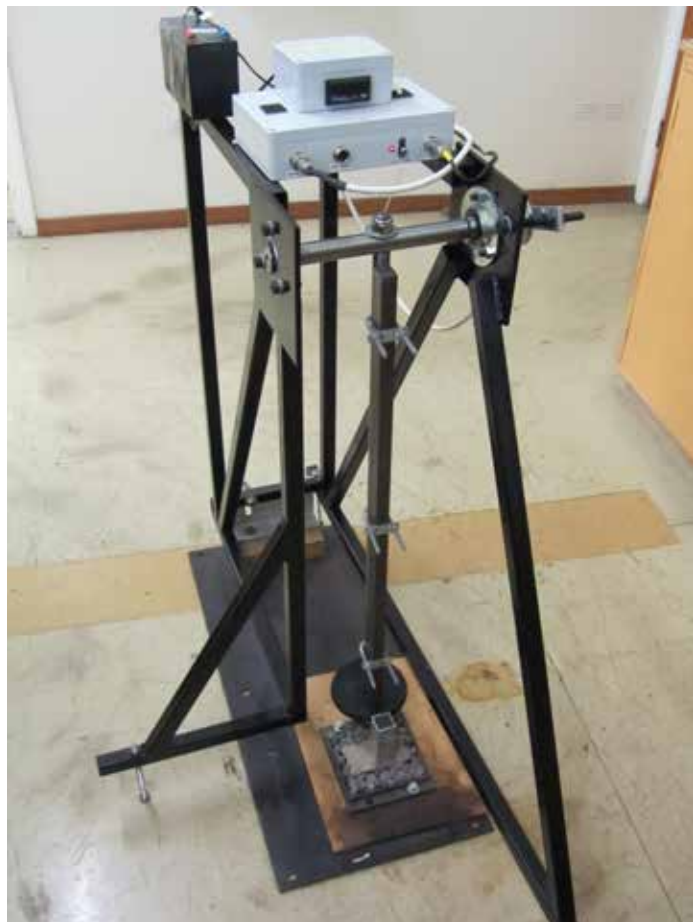
Pendulum apparatus for measuring seal cohesion (specimen in place)
