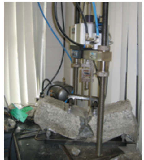
Test set-up for measuring flexural beam properties, with the beam at breaking point after the initial test
