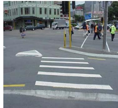
*No tactile paving at the end of this pedestrian crossing. Note lack of dropped kerb in the central island.*
