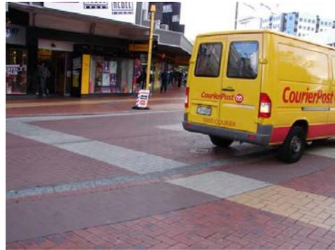
*Poor colour contrast between the footpath and the road. Note courier van parked half on the road/half on the pavement in the middle of a pedestrian crossing.*
