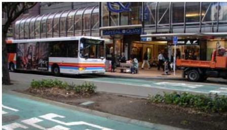
*Crossing desire line(from a side road) has worn out the planting in the central median*
