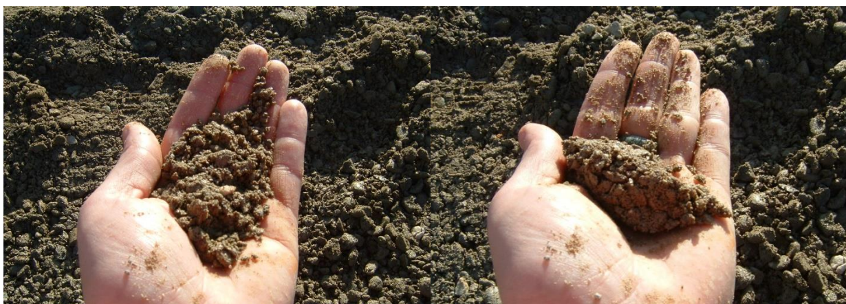
Figure 3: Take a handful sample of material and remove all particles greater than 5mm as the water generally held by the fines / sand fraction. Squeeze the sample in your hand. If it holds together well, the material is close to OWC.
