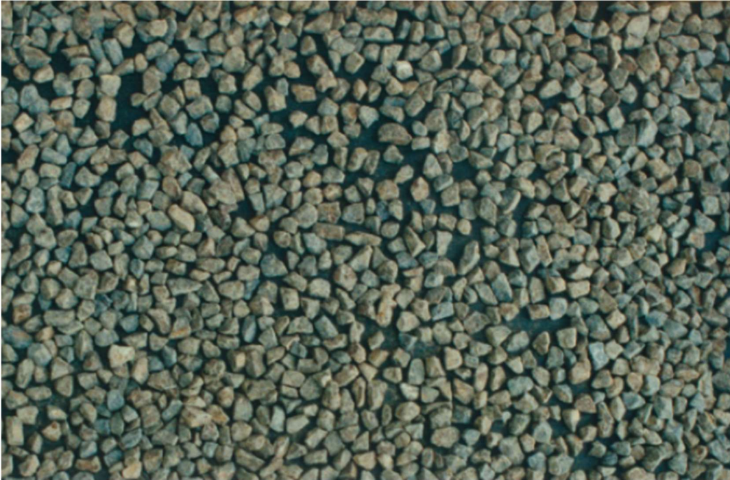
Figure 1: Typical chip application for a first coat seal.
