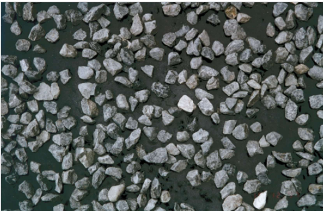
Figure 2: Typical chip application rate for the first layer of a racked-in seal.
