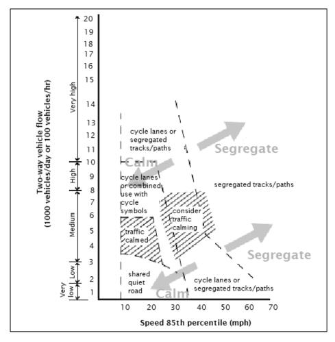
Figure 2.2 Cycle facilities based on motor traffic volumes and speeds (adapted from Transport for London 2005)
