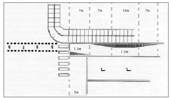
Figure 2.4 Layout with narrowed cycle lane and marked cycle crossing (Jensen 2000a)
