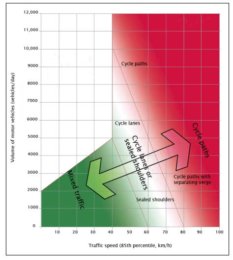
Figure 2.1 Preferred separation of bicycles and motor vehicles according to traffic speed and volume (adapted from LTNZ 2004)
