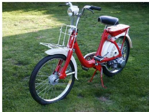
Some mopeds, such as the Honda shown in figure 2.9, were effectively hybrids. This Honda has a power output of 900W, a top speed of 40km/h, and a claimed fuel consumption of 90km/l. Note that in both cases, the claimed fuel consumption and speed are for engine-only operation.
