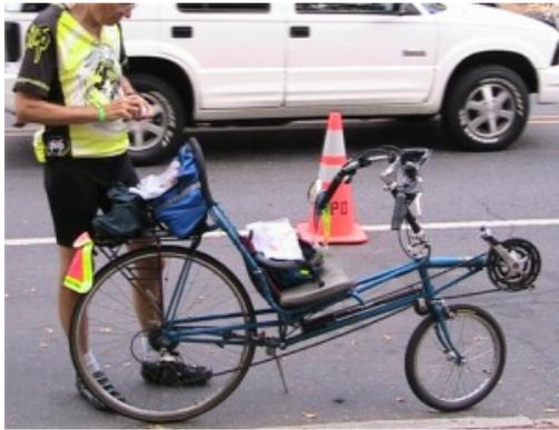
Figure 2.3 Easyracer long wheelbase recumbent (de Pont)
