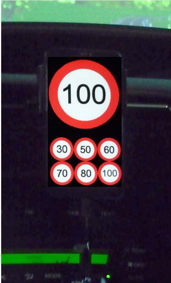
Speeding (defined as exceeding the speed limit by 4 km/h or more for at least three seconds) was accompanied by the main speed rondel flashing on/off (each state 0.5 second) until the participant reduced their speed to within 4 km/h of the speed limit. For the audio visual conditions the flashing rondel was accompanied by a beep, synchronised with the flashing, until speeding stopped.
