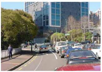
Pruning of the lower branches would allow the traffic signals to be clearly seen. Crash reduction studies carried out in Auckland City regularly find similar faults over the entire roading network.
