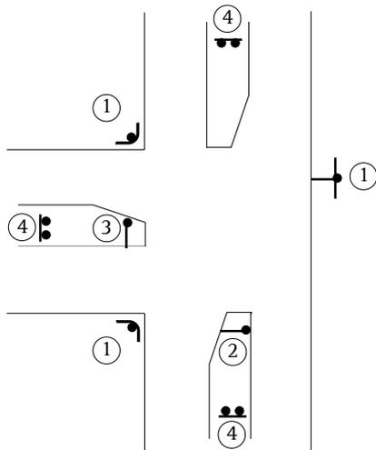
Signs for both arterials should be provided at positions (1). An additional side-road sign may be provided at position (2). If the name of the through route changes an additional sign may be provided at position (3).
