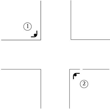
A sign showing the name of each street at position (1) is sufficient, unless the names of one or more streets change, in which case an additional sign or signs should be provided at position (2).
