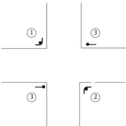
Minor street and arterial names should be provided at positions (1) and (2).
