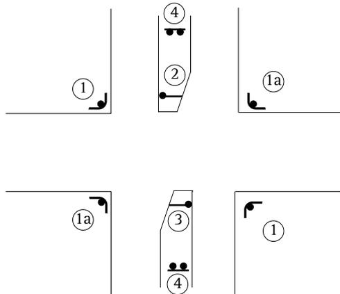
Street name signs for the divided arterial should be provided at positions (1) or (1a). Where the minor street name is the same on both sides of the intersection, street name signs should be provided at positions (1) or (1a). If the street name changes, additional signs may be provided at positions (2) and (3). Advance street name signs should be provided at position (4) for major side-roads.
