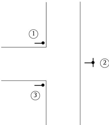
The name of the side street should be provided at position (1) and the name of the through street at position (2).
