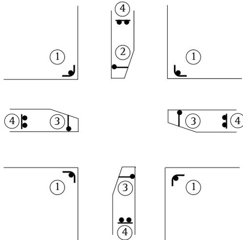
Signs for both arterials should be provided at positions (1). If either street name changes, additional signs may be provided at positions (2) and/or (3) as appropriate. Advance street name signs should be provided at positions (4).
