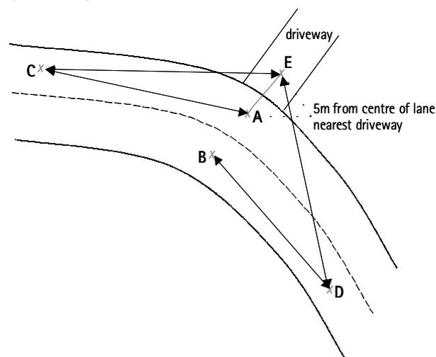
Points A, B, C and D are as shown in Figure 6.2, with points C and D established by measuring the sight distance from Table 6.1 along the centre of the appropriate lane from points A and B.
