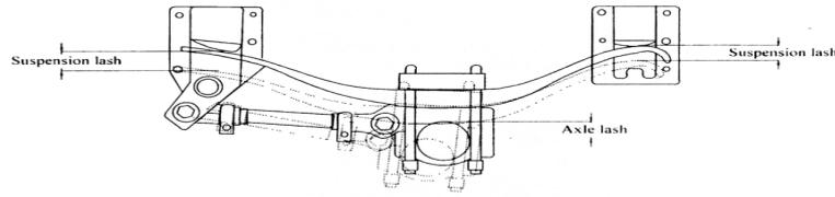
**Figure 3 Illustration of suspension and axle lash**
