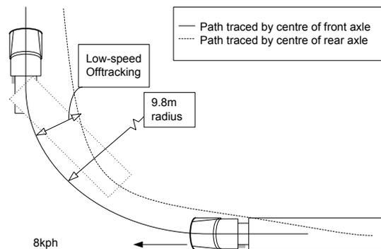
Figure 1 Low-speed Offtracking
