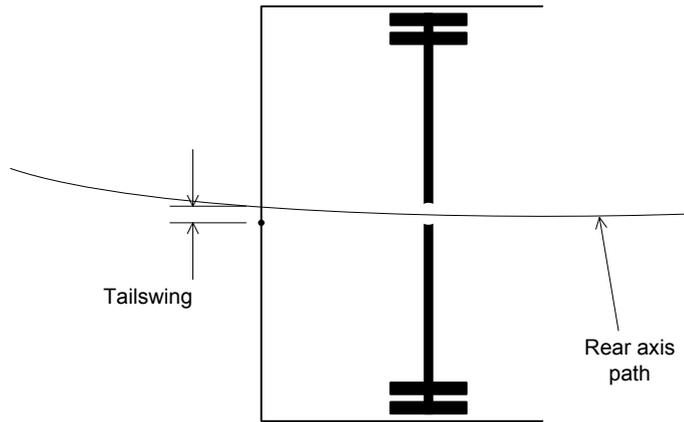
Figure 3 Tailswing of vehicle during 12.5 m radius turn
