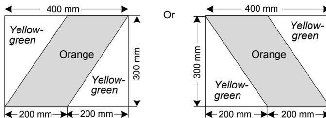
**Figure 1 Minimum dimensions of hazard warning panel** [Refs. 2.1(4)(b), 6.10(1)(c) and (d)]
