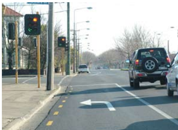
Figure 18 No safe and legal waiting position for straight-through cyclists during left-turn-only phase
