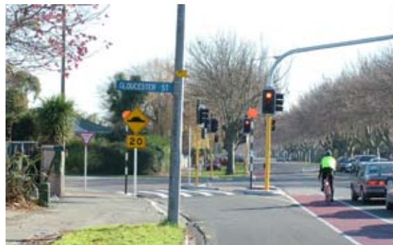
Figure 6 Slip lane with zebra crossing on raised platform for speed control
