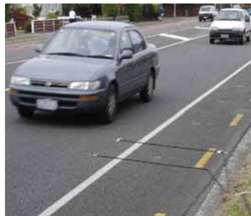
Figure A3 Tubes extend 400 mm beyond the cycle lane or edge line
