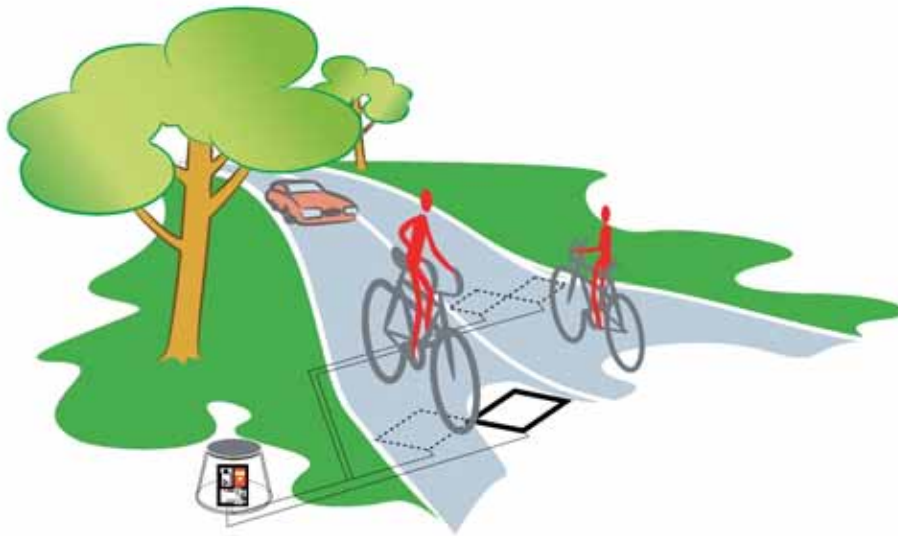
Figure 11 How Eco-Counter's ZELT inductive loop sensor system works
