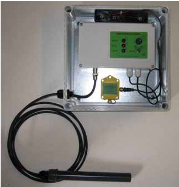
Figure 6 Chambers Electronics' Bike and People Counter
