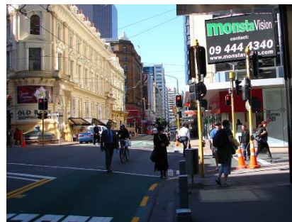
Figure 6.5 Inappropriate use of variable message sign as it is located at busy city intersection
