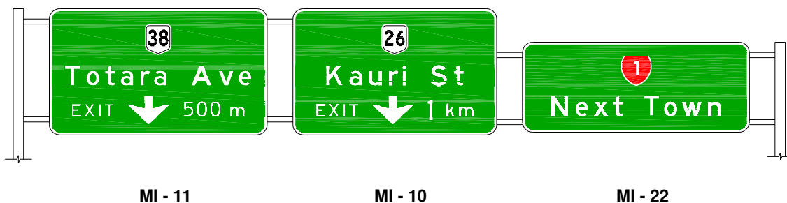
FIGURE 2.4: TYPICAL SECOND ADVANCE EXIT SIGN ASSEMBLY FOR THE FIRST EXIT WHEN EXITS ARE LESS THAN 800 m APART
