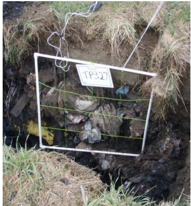
Figure 6.1. An example of a test pit where rubbish was encountered below the surface.
