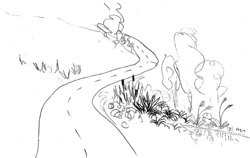
Figure C.8 Sketch of treatment wetland and swale leading to stream, capturing stormwater runoff from adjacent road. It comprises sedges, rushes, tussocks and reeds in the wettest seepage areas then swamp forest shrubs and trees in ephemerally wet sites
